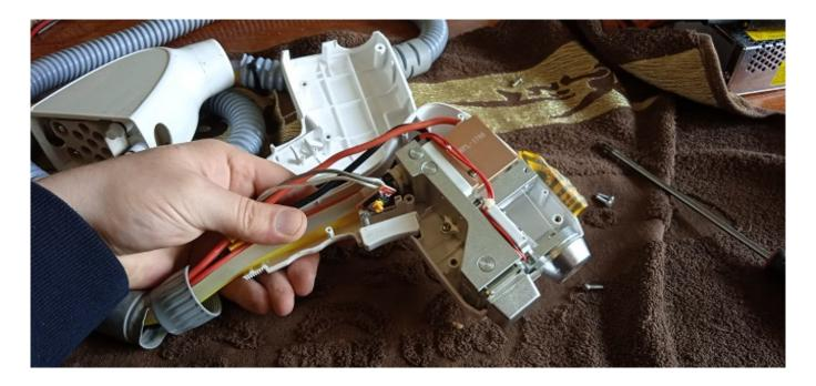
Replacing and setting up 808nm diodes in the manipules of epilation lasers.
