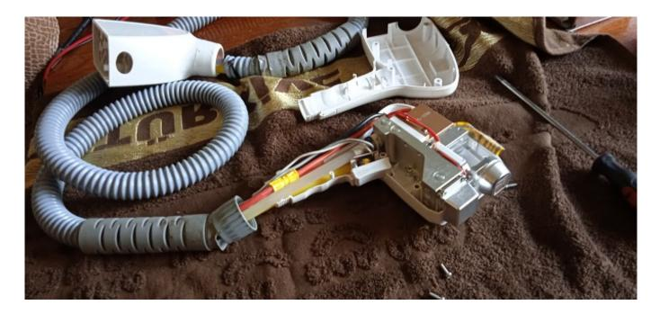
Repair of diode pens 808nm with the installation of new bars on order.
