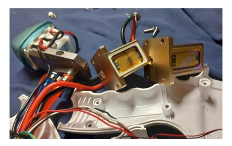
A full cycle of maintenance of laser handles 808NM: from diagnosis to bars replacement.
