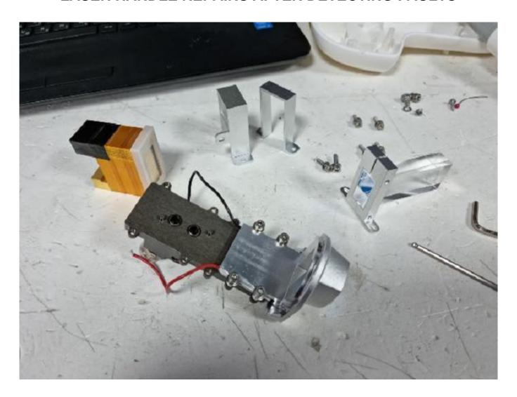
Installation of new bars 808nm in laser handles, repair of all brands.
