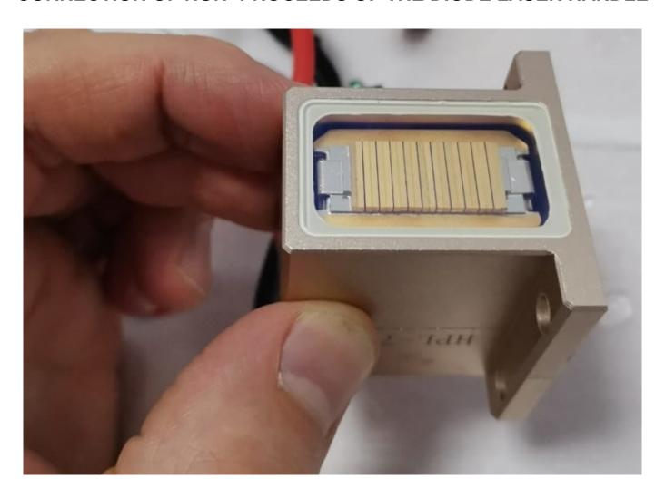
Maintenance of laser manipula 808nm. Bar with a capacity of up to 1600 watts.
