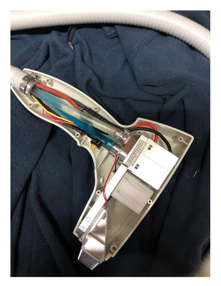
Repair of diode lasers 808nm with a replacement of bars to order.
