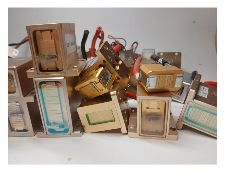
Manufacturer of laser components - 1000W LST & DVS stacks
