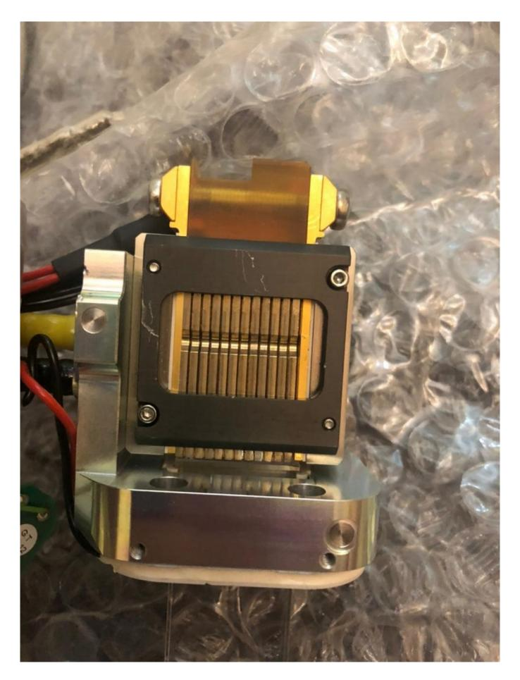
Replace faulty bars in 808nm manipules from different manufacturers.
