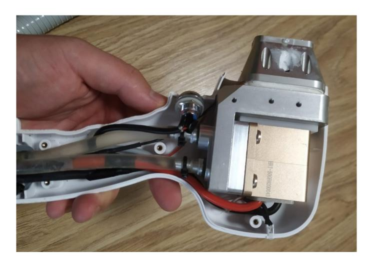
Restoring the manipulus of diode lasers 808NM, installation of bars up to 1600W.
