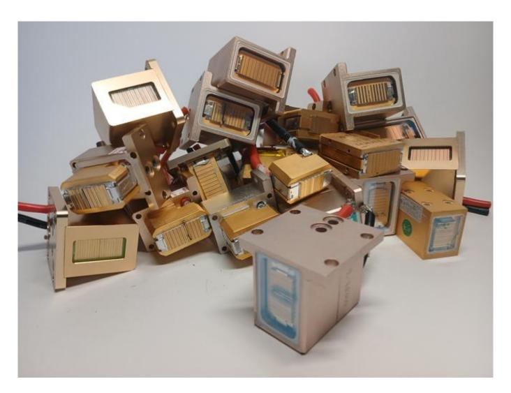
Parts for repairing a laser of hair removal without flashes
