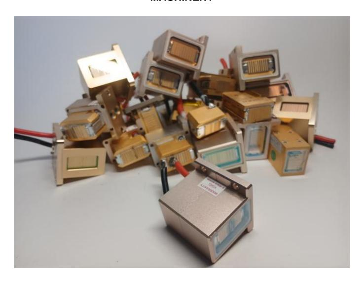
The principle of the diode stack in the laser handle
