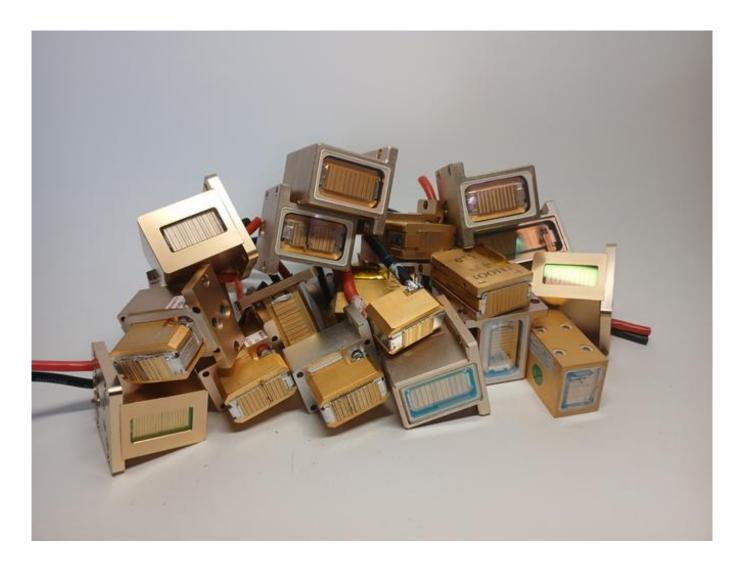
Components for laser repair with faulty flashes
