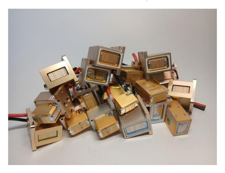
Explanation of the term "diode stack" in the laser handle
