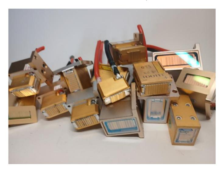
Why is diode stack used in the diode laser manipul?
