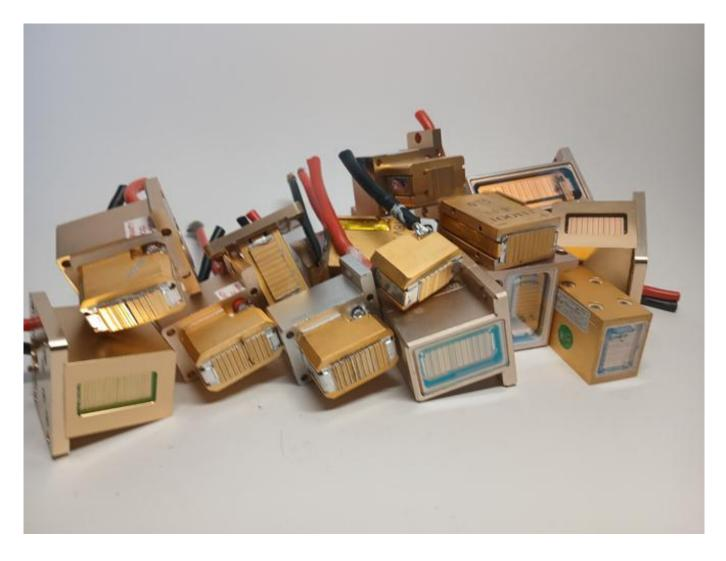
What is a diode stack in the laser handle for hair removal?
