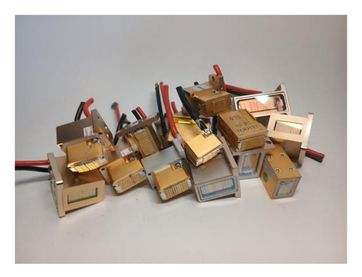
Spare parts for repairing the laser of hair removal during flashes breakdown
