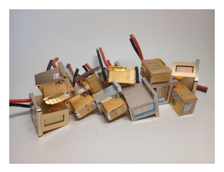
Spare parts for the restoration of the laser in the absence of flashes
