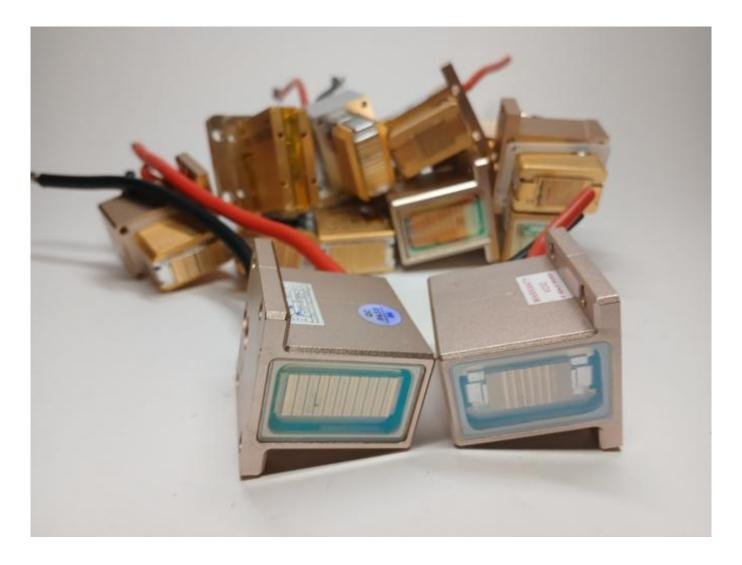
Spare parts for a laser of hair removal with a malfunction of the outbreaks
