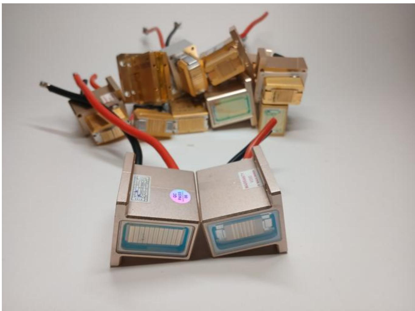
Set of diode laser handle modules
