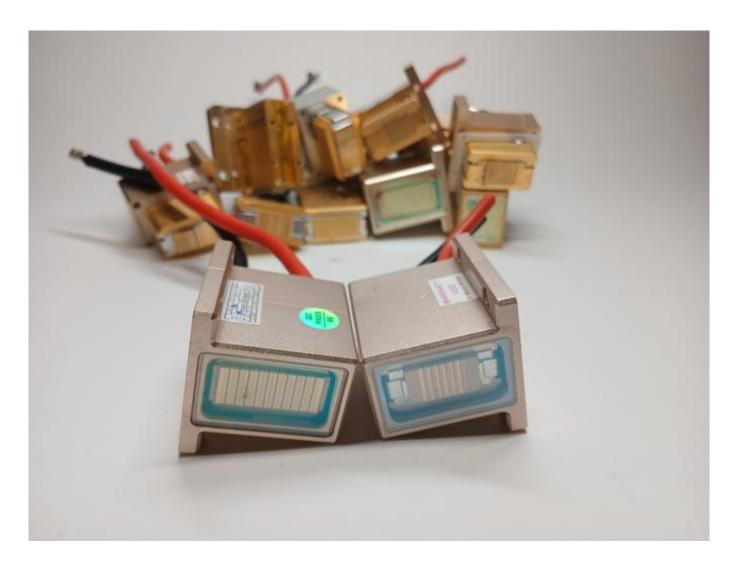
Parts for replacement in a laser handle
