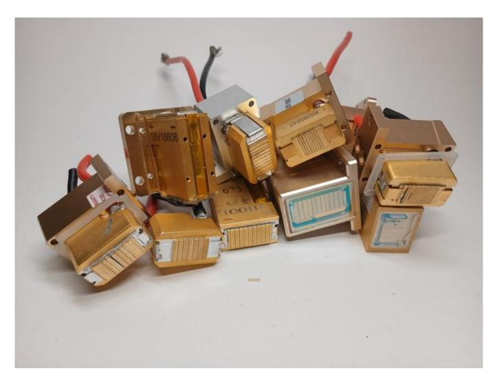
Electronic elements for repairing a laser handle
