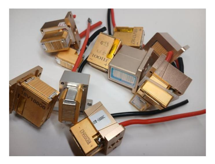
Exchange modules for a diode handle
