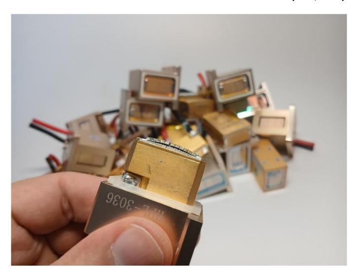
Spare parts for laser repair in case of malfunction of flashes
