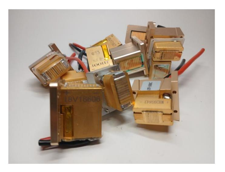
Replaced nodes for a diode laser handle
