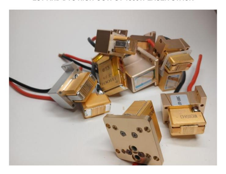
Set of spare parts for a diode laser handle
