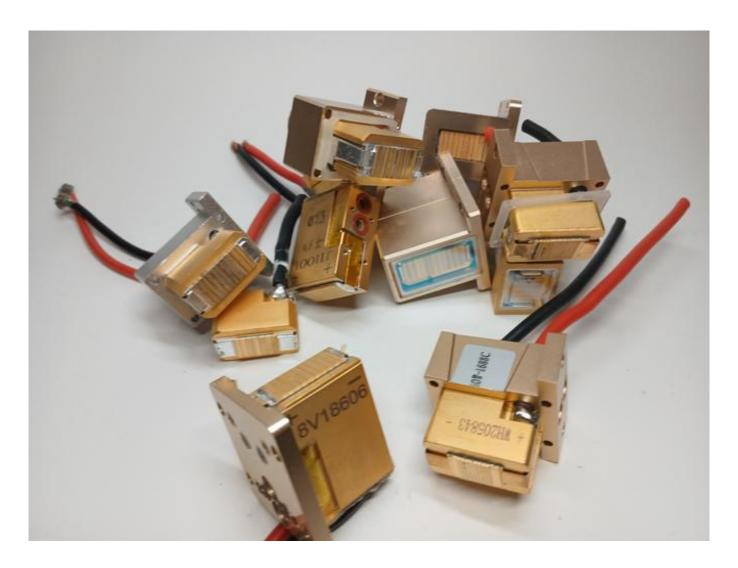
Elements for repairing a diode laser handle
