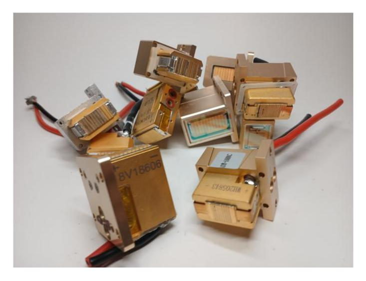
Components for restoration of a laser handle
