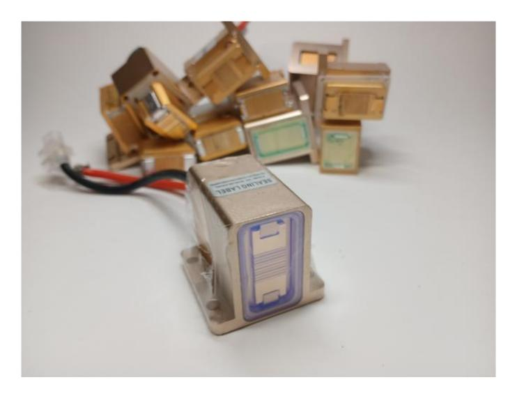
The hardware part of the diode laser handle
