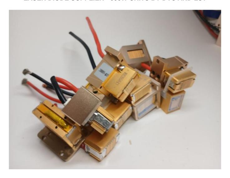
Spare parts for diode laser handles
