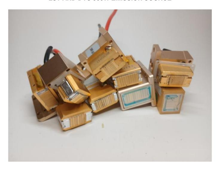
Spare parts for the laser handle 808 nm
