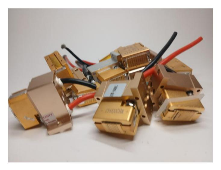
Radiators and coolers of a diode laser handle
