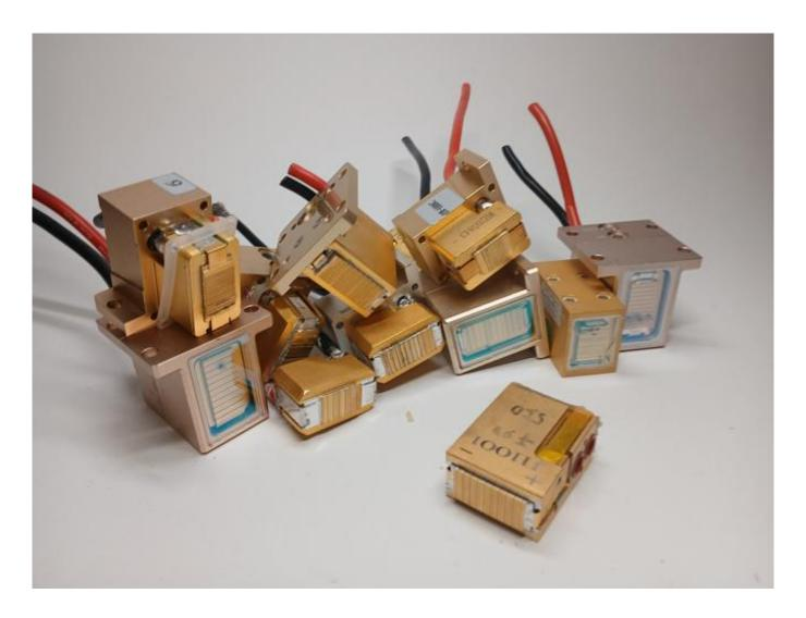
Replaced parts of the handle of the cosmetology laser
