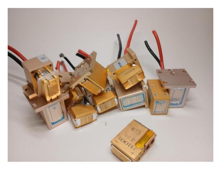
Working elements of a diode laser handle
