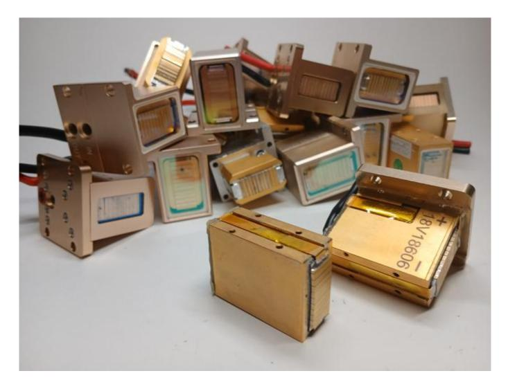
Laser block for the handle of the cosmetic apparatus
