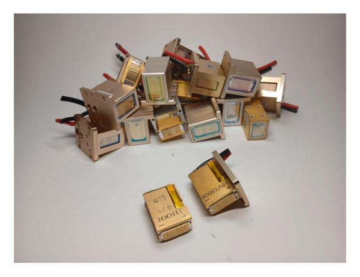
Diode matrix for the handle of the epilation apparatus
