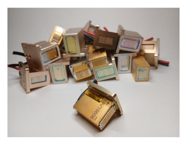
Diode emitter for the handle of a cosmetology device
