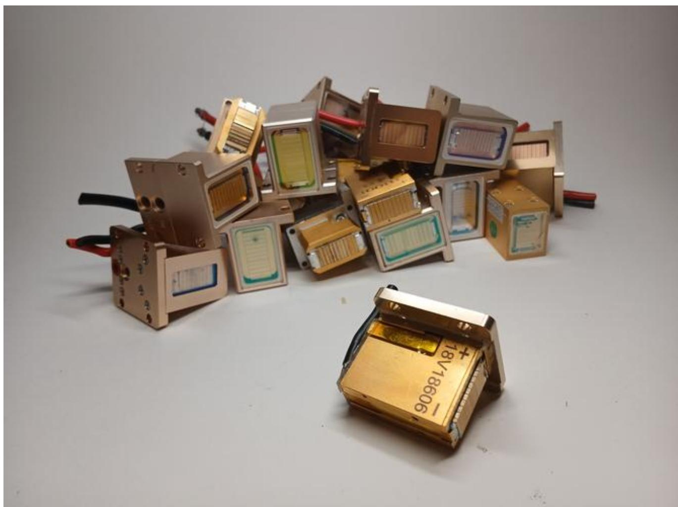
Diode module for the handle of the epilation device
