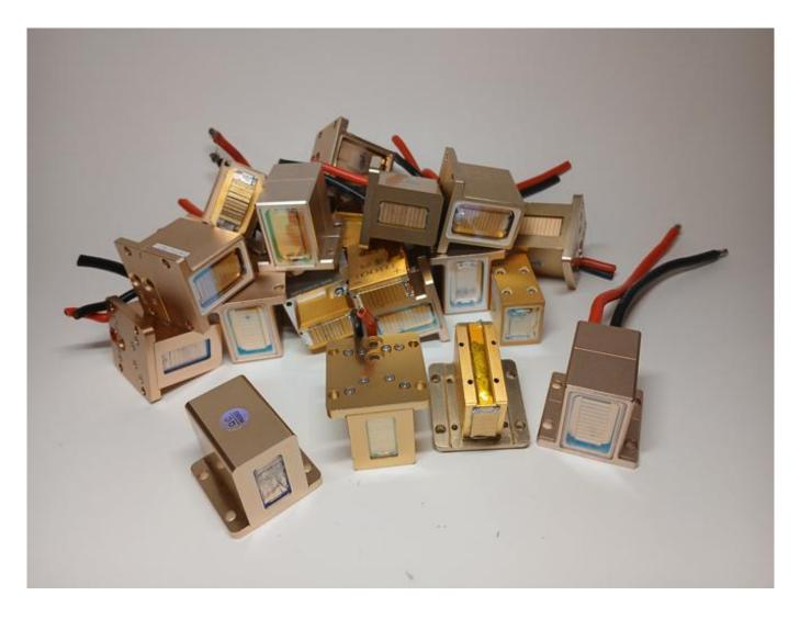
Laser stack for the handle of the epilation device
