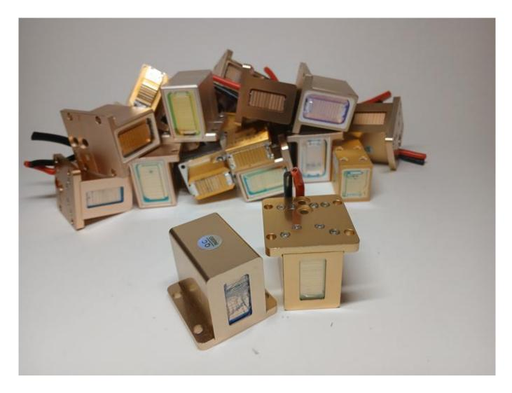
Diode glass for the handle of the epilation apparatus
