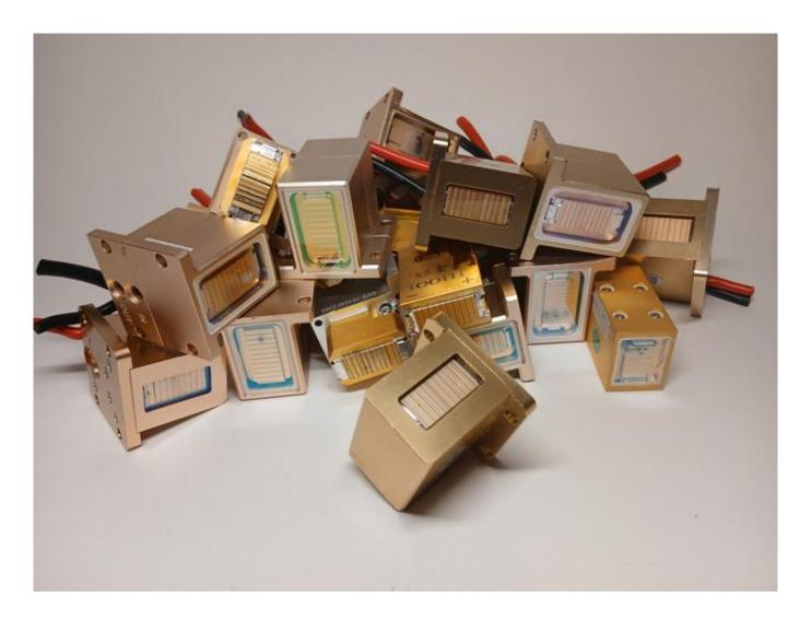
Diode block for the handle of a cosmetology device
