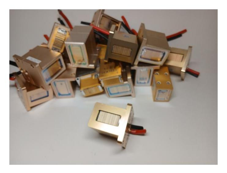
Diode emitter for the handle of the epilation device
