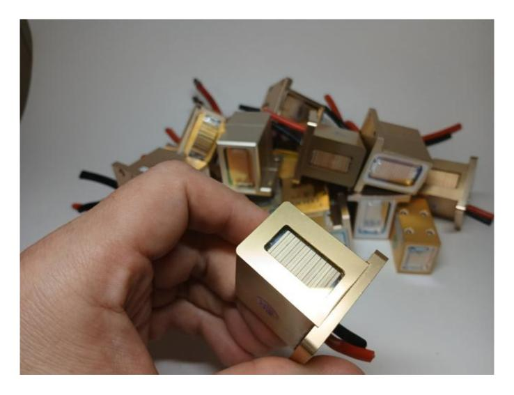
Laser module for the handle of the epilation device
