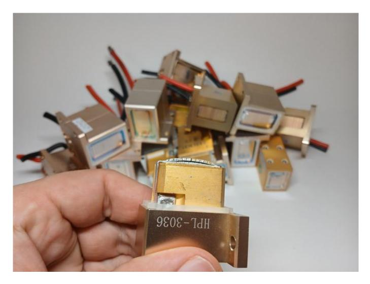
Diode module for the handle of the laser of hair removal
