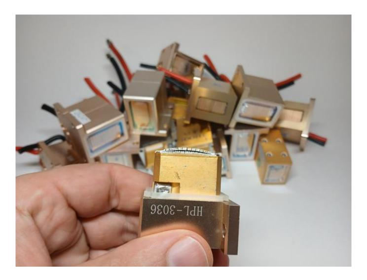
Laser radiating element for the handle of a cosmetological laser
