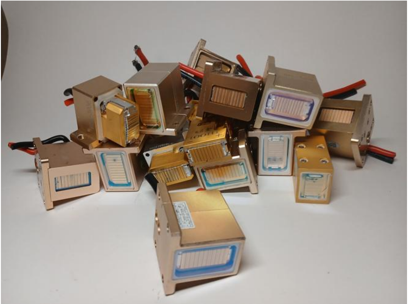
Diode cassette 808 nm for epilator handle
