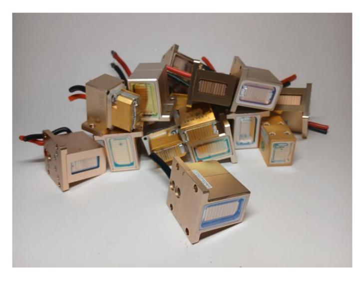
Diode block for the handle of a cosmetic device
