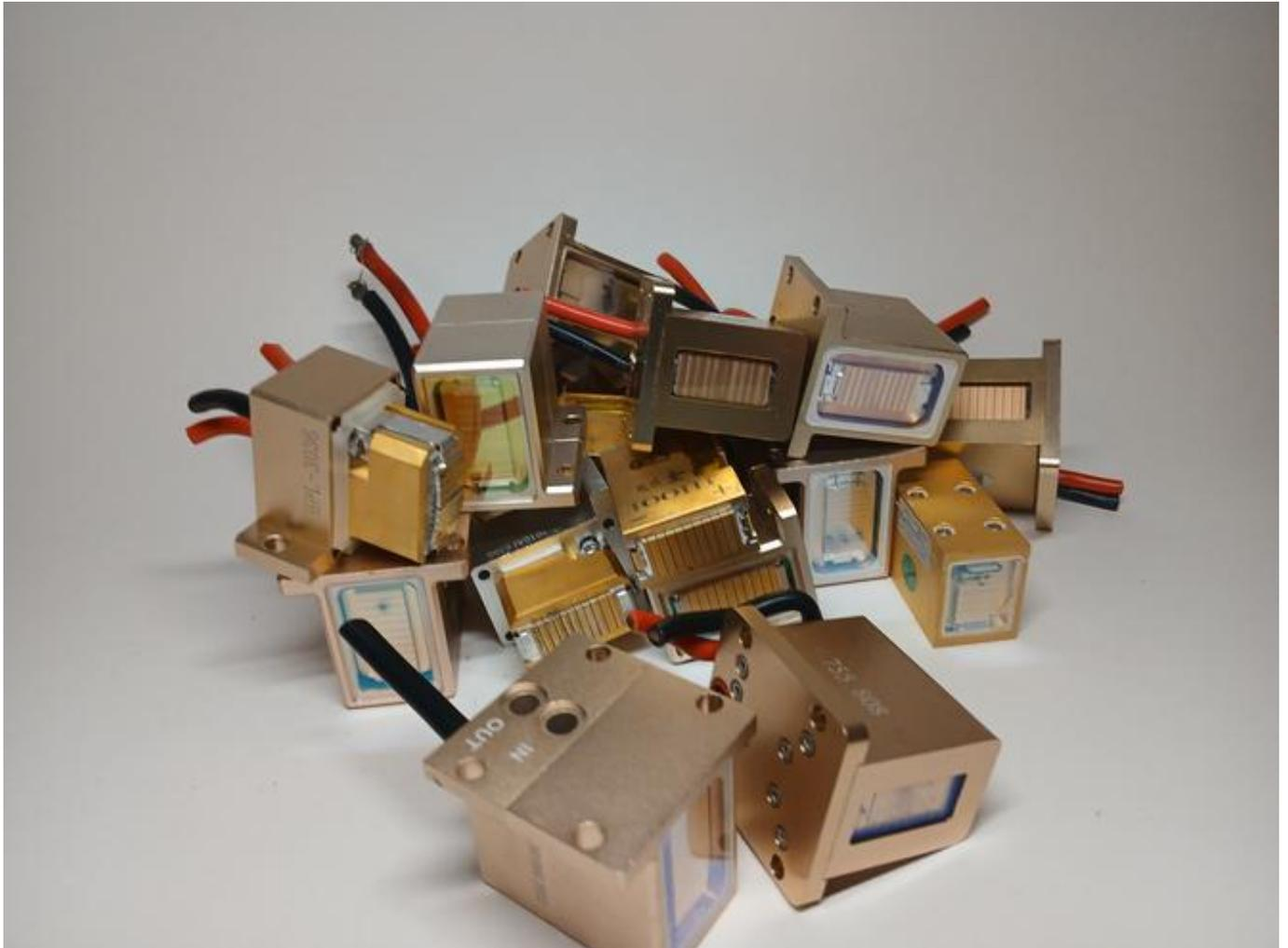
A set of diodes for the manipula of the cosmetology apparatus
