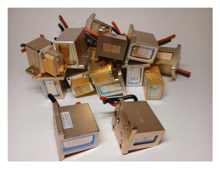
Laser emitter for the handle of a cosmetology device
