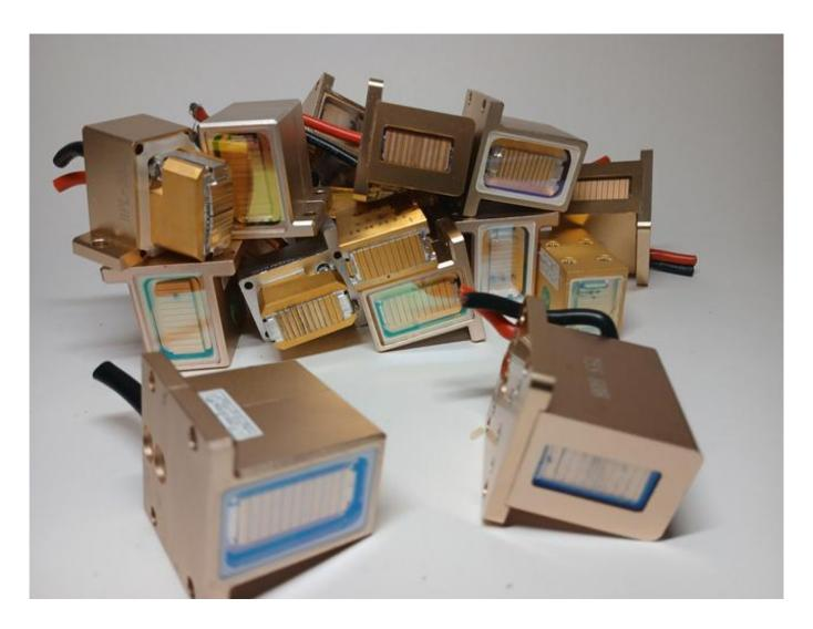
A set of diodes for the laser manipula
