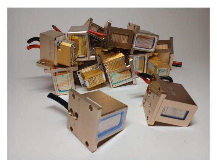
Laser module for the handle of a diode epilator
